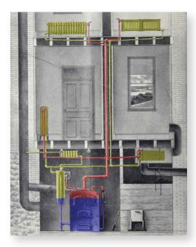
A popular heating system from the early 20th Century was the "vapor" system, which was designed to operate with very low pressure steam. The inventor of the first vapor system was Albert Broomell, who manufactured and sold his system components through the Vapor Heating Company. They can still be found operating today, although many are not functioning as designed because of inappropriate modifications.
