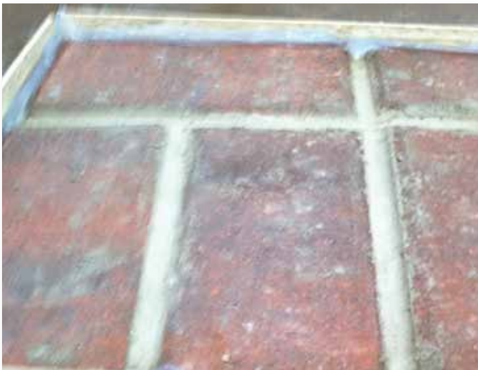
BEFORE AND AFTER PHOTOS OF NATURAL CEMENT MORTAR 1:1 WITH AMENDMENT AFTER 50 FREEZE-THAW CYCLES.
