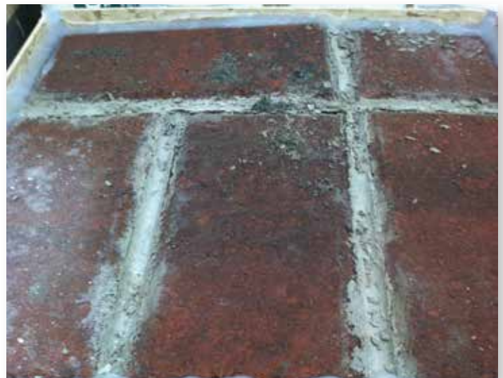
BEFORE AND AFTER PHOTOS OF NATURAL CEMENT MORTAR 1:1 WITHOUT AMENDMENT AFTER 3 FREEZE-THAW CYCLES.
