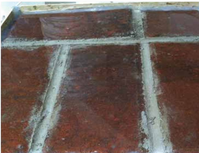
BEFORE AND AFTER PHOTOS OF NATURAL CEMENT MORTAR 1:1 WITHOUT AMENDMENT AFTER 3 FREEZE-THAW CYCLES.
