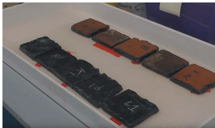
Capillary suction test of brick sections with and without an air barrier on the exposed top. Photo Credit: Simpson Gumpertz & Heger Inc.
