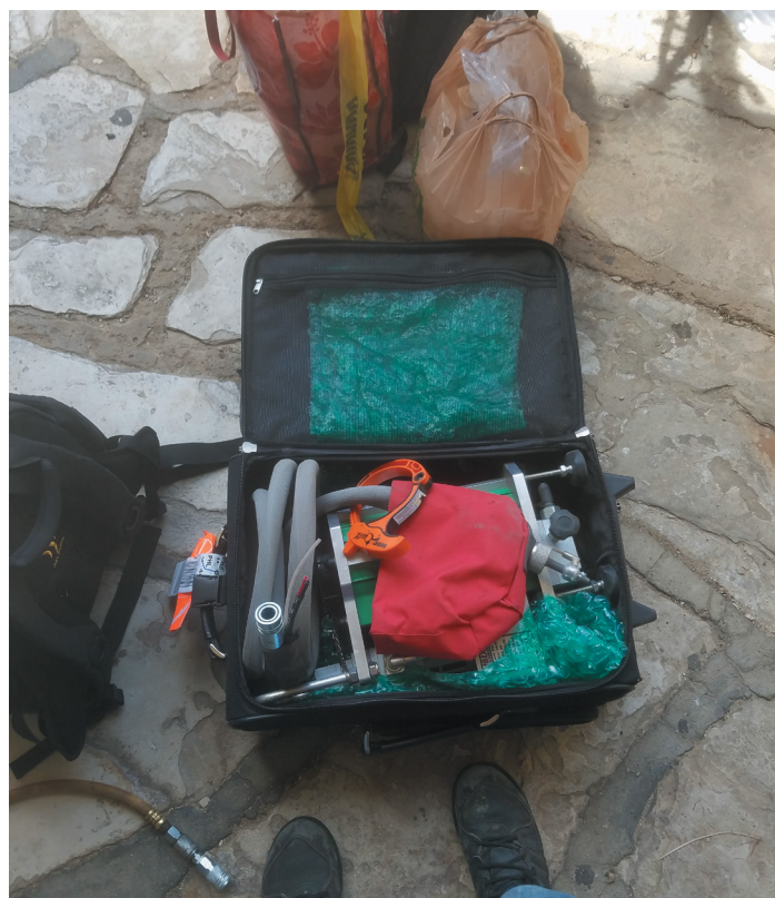
Blast cleaning unit in a Suitcase, Santa Barbara Courthouse. Photo credit: Ken Follet
