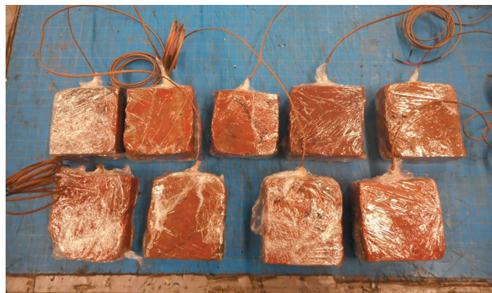
Brick samples prepared for freeze/thaw cycling. Photo Credit: Simpson Gumpertz & Heger Inc.
